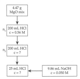
$n(NaOH) = 0.05 \times 0.00986$ =  $4.93 \times 10^{-4}$  mol 1:1 ratio :: n(HCl)=  $4.93 \times 10^{-4}$  mol in 25 mL :: in 200 mL n(HCl)=  $4.93 \times 10^{-4} \times \frac{200}{25} = 3.944 \times 10^{-3}$  mol
