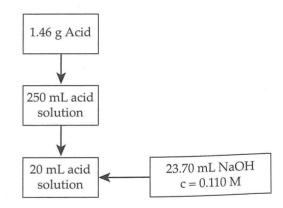
$$\begin{split} n(NaOH) &= 0.110 \times 0.02370 \\ &= 2.607 \times 10^{-3} \ mol \\ Ratio \ of \ acid \ to \ NaOH = 2:1 \\ n(Acid) &= \frac{1}{2} \times n(NaOH) \\ &= 1.3035 \times 10^{-3} \ mol \ in \ 20 \ mL \\ In \ 250 \ mL \ n(Acid) &= 1.3035 \times 10^{-3} \times \frac{250}{20} \\ &= 0.01629 \ mol \\ M_r &= \frac{m}{n} = \frac{1.46}{0.01629} = 89.6 \ g \ mol^{-1} \end{split}$$
